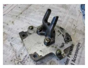
This might be a good time to back up and review what "neutral" is. When the sliding sleeves for gears 1/2, 3/4, and 5/R are all in their middle positions the transmission is in neutral. After the 5th/R gears have been removed neutral can be checked without looking inside the center housing. You will see two shafts, to the left of the pinion shaft, which protrude into the nose cover's chamber.
