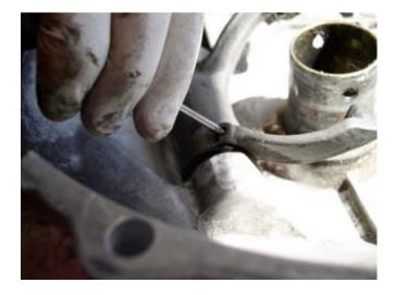
When you drive out the release fork pin be sure to hold the fork at the pictured angle, otherwise you will drive the pin into the aluminum below the fork. Once the screws are removed from the TOB (throw out bearing) guide tube, use your mallet to gently tap the tube from inside the housing. It has an o-ring so it might take a few taps.
