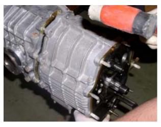
To remove, place your left hand under the housing and gently pull it off; the shift rod will come with it. Set the housing aside and check out 1st-4th gear sets! Depending why your transmission is apart this is when you usually find most of the carnage. Our subject transmission is a pleasant surprise, at first glance I see bad dog teeth on 1st, worn synchro rings, and...not much else!
