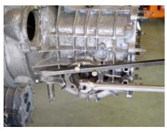
Once the flanges are removed the differential side cover will come off. Remove all of the 8mm (13mm wrench size) nuts, and use a soft mallet to tap against the small overhangs provided.
