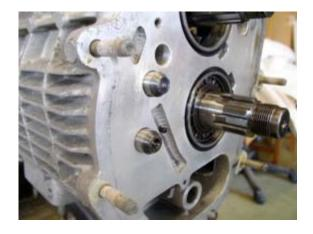
If the two shafts appear as pictured the gear cluster inside the housing is in neutral. If one shaft protrudes about 10-12mm further than the other, or if the tip of one shaft sits approximately flush with the housing, the transmission is in gear.
