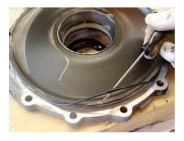
...and use a punch or large screwdriver to remove the flange seal (support the cover on a couple short pieces of 2x4).
