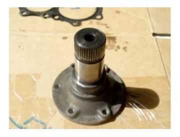
Put the remaining axle flange into the differential carrier, and snug down the bolt for it by hand. Use the flange to lift the carrier/ring gear assembly out of the housing and place it on the other axle flange.
