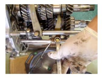
Remove the 3/4 shift rod detent and spring by removing the upper threaded plug on the side of the differential housing.
