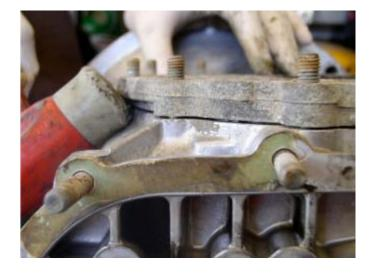
Care must be taken to watch the cover as it lifts away from the housing because it can easily get cocked to one side, which might cause damage. Sometimes the side cover is extremely tight, patience is your friend. Work slowly until it comes free from the housing. Use a dentist's pick, or similar, to remove the o-ring...
