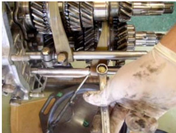
Remove the 3/4 shift rod detent and spring by removing the upper threaded plug on the side of the differential housing.
