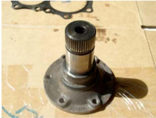
Put the remaining axle flange into the differential carrier, and snug down the bolt for it by hand. Use the flange to lift the carrier/ring gear assembly out of the housing and place it on the other axle flange.
