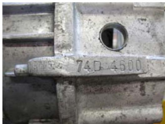
1972 through early production 1977 models had magnesium housings (cases); all later 915s had aluminum housings. 1972-75 models used a mechanical drive for the car's speedometer, replaced with an electronic unit in 1976. 1972-74 versions were the only 915s fitted with a 7:31 ring and pinion ratio. The above type-numbers might carry over, or carry back, to another model year; sometimes with Porsche nothing is certain.
