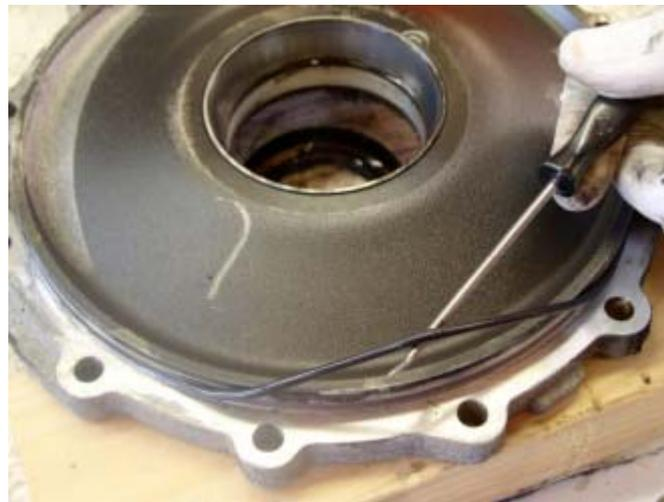
...and use a punch or large screwdriver to remove the flange seal (support the cover on a couple short pieces of 2x4).
