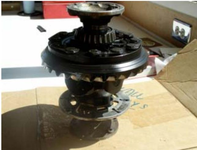
Why place the diff on the flange? Never set anything, these parts are heavy, on an unsupported bearing, which could damage the bearing (you might choose to re-use the carrier bearings).
