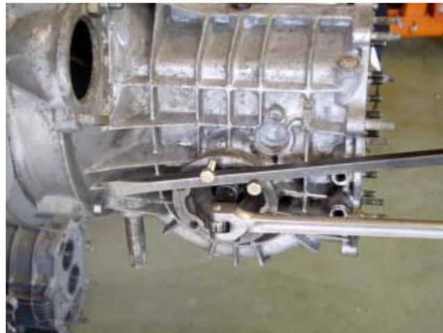
Once the flanges are removed the differential side cover will come off. Remove all of the 8mm (13mm wrench size) nuts, and use a soft mallet to tap against the small overhangs provided.
