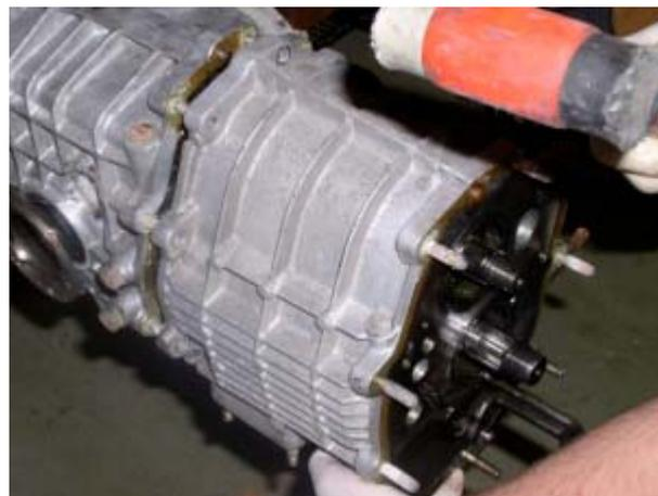
To remove, place your left hand under the housing and gently pull it off; the shift rod will come with it. Set the housing aside and check out 1st-4th gear sets! Depending why your transmission is apart this is when you usually find most of the carnage. Our subject transmission is a pleasant surprise, at first glance I see bad dog teeth on 1st, worn synchro rings, and...not much else!
