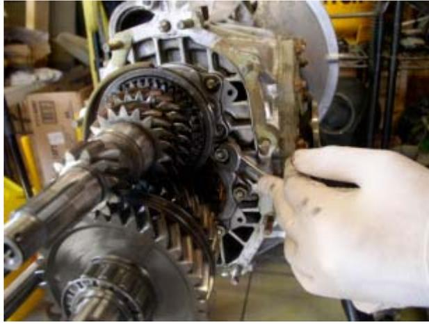
It's a good technique to loosen the nuts with the box end of your wrench, then remove them with the open end of the wrench.
