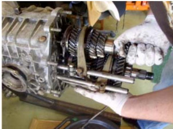
After gear cluster removal the pinion depth shims, see the next picture, can be carefully removed.
