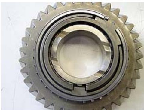
NOTE: The synchro ring for first gear is unique in that it has a groove in its two flat sides. Early rings had the groove located closer to the middle of each side; late versions have the groove as pictured above.
