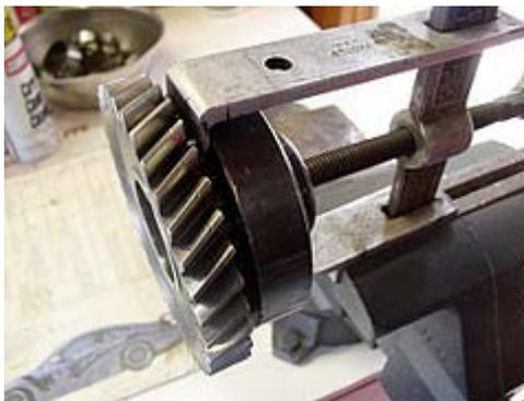
Even though a puller is designed to pull with equal force (a three jaw puller might be a better alternative than what I use, but I'm used to it), watch closely to be sure that the ring doesn't get cocked to one side.
