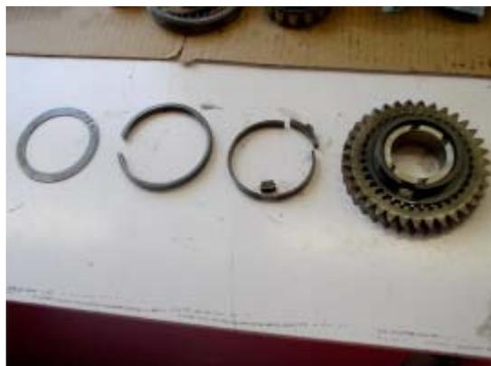
Only the retainer ring and the dimension of the installed synchro are shared with 2nd gear.
