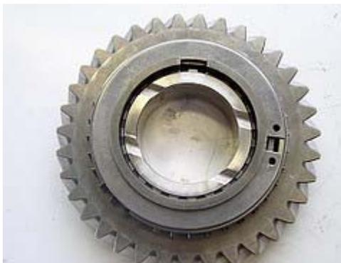
Be sure to rotate the retainer to the approximate position shown, placing the opening in the retainer away from the opening in the dog tooth ring and the opening in the synchro ring. Measure the synchro ring.
