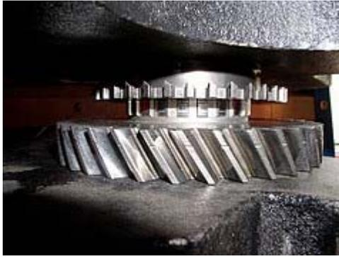
Don't worry, the above picture is playing tricks, the dog teeth are perfectly "square" to the gear. From that point simply activate the press, but watch your parts to be sure they stay aligned. If the ring gets off-center slightly, and get's cocked over, the press can easily split the ring. At that point you will throw about \$200 into the trash can.
