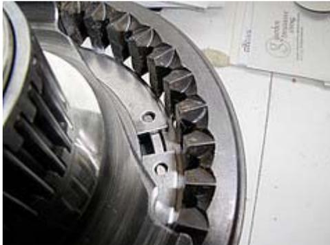
The asymmetrical teeth must face up, toward 1st gear. The asymmetrical teeth are on the same side as a machined groove on the O.D. of the slider...
