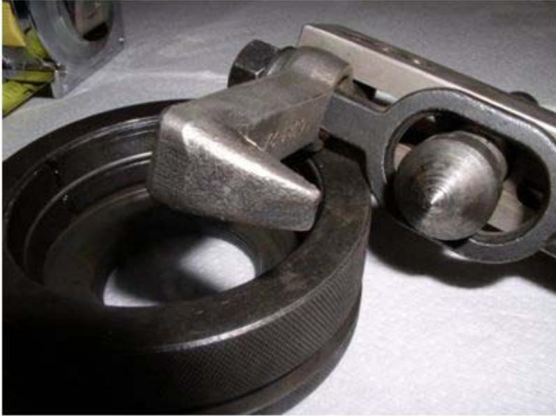
Set up the puller, and insert a steel puck for the center post of the puller to push against...
