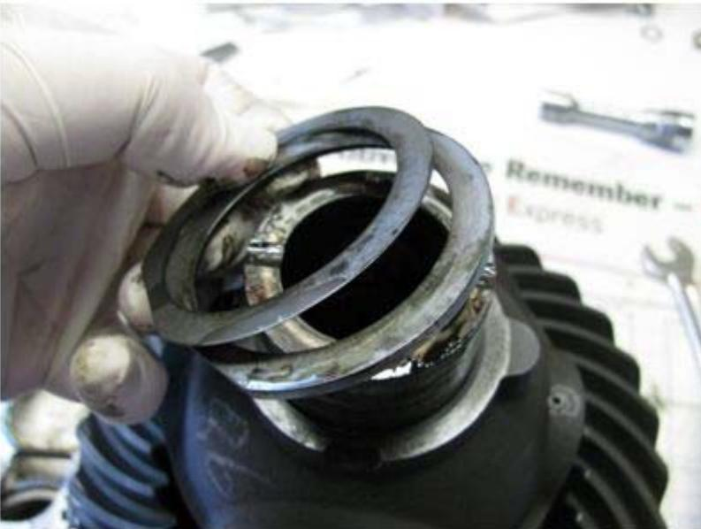
Notice that there are two shims, the thin one is .25mm (for fine adjustments); the thicker one is usually about 2.7mm - 3.1mm (available in 1.0mm increments from 2.4mm to 3.7mm).
