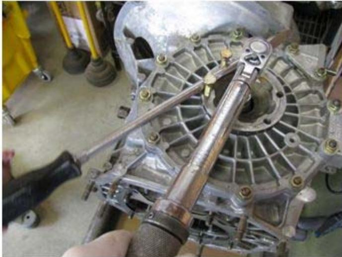
NOTE: Axle flange bolts changed during 915 production, always verify the type used on your differential, and look up the torque spec for them.
