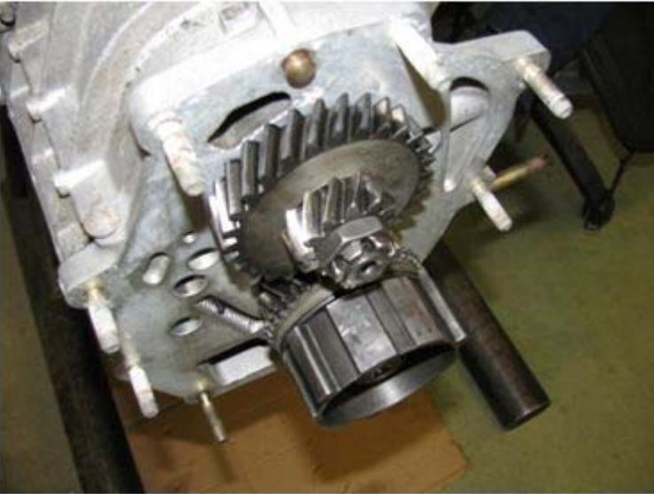
...engage the slider with 5th gear...
