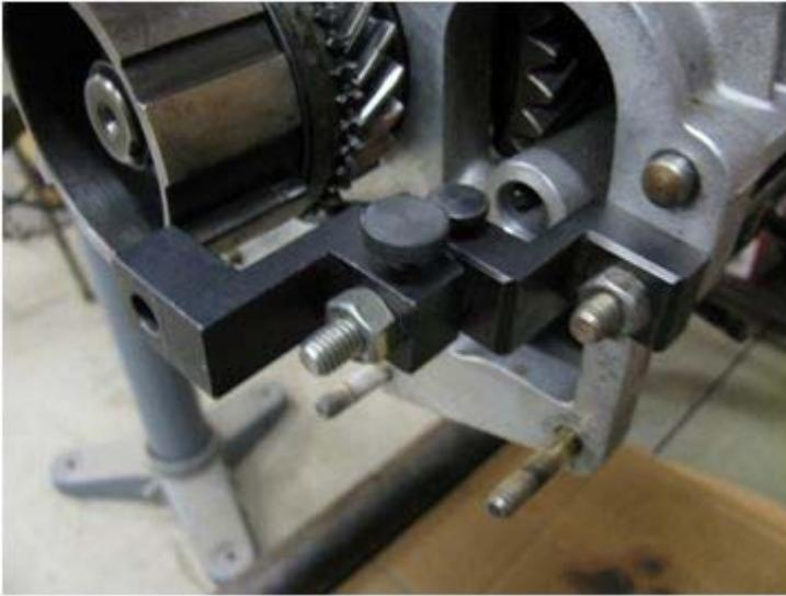
The movement in the pinion shaft is the clearance between the loose gears and fixed gears on the two shafts, and all of that movement must be eliminated.
