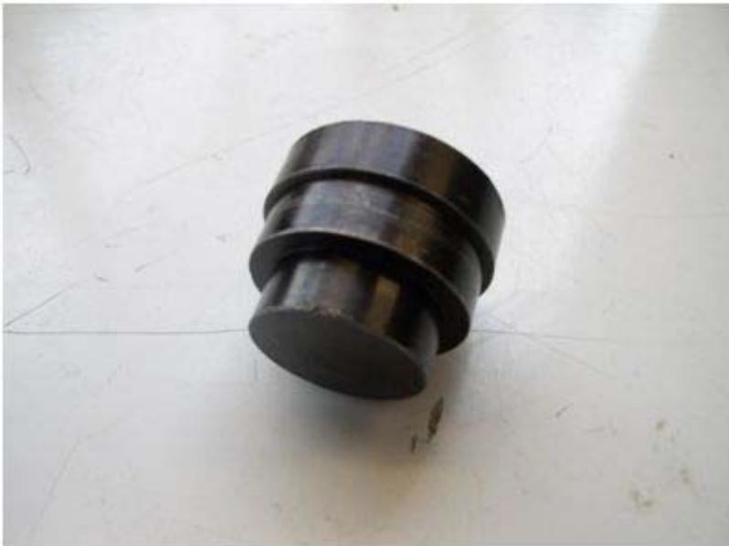
...into the hole, in the center of each carrier bearing, that the axle flange fits into. The puck measures 30mm (length) x 37.6mm (diameter) x 34.8mm (1st step) x 31mm (end step). As you remove the bearing on the speedo sensor side be aware that the magnet ring will come off before the shims.
