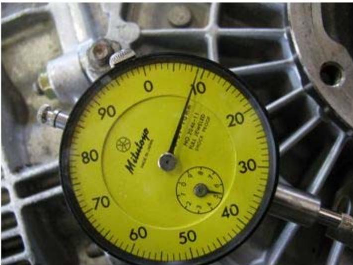
That means that increasing shim thickness at the side cover bearing does more than increase the pressure against the side cover, it also applies pressure against the ring gear, which actually pushes the ring gear closer to the pinion head. So much for the theory!
