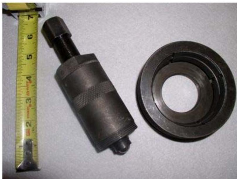
...is available to remove bearings, but a high-quality puller with the correct length jaws will also work.
