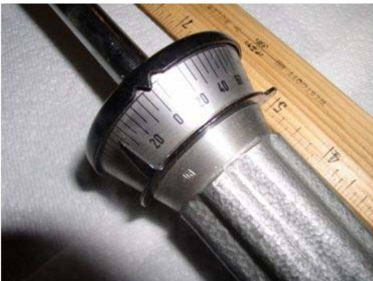
My washer is slightly oversized on the OD, so I had to bevel the outer edge for clearance; I'll explain this
