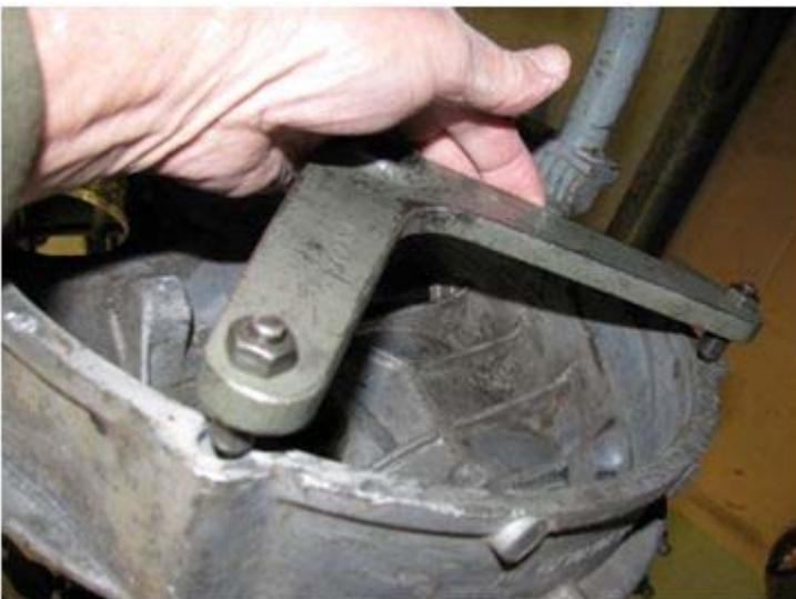
...and install and torque the old collared nut. The torque spec is 181 lb/ft.
