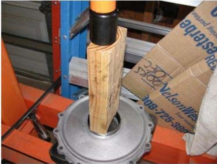
The important thing to remember is to keep the bearing race perpendicular to the housing/cover; damage can occur if the race gets cocked to the side. (Application of heat is acceptable if needed). Also, knowing when the races are all the way in and seated can cause doubt, but checking them is easy. Just flip over the housing/cover and look into the axle flange opening; the race will show a gap if it's not seated. These are in all the way:
