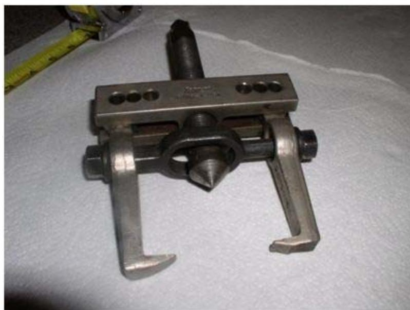
Actually, a puller is necessary on the speedo sensor side (915s equipped with electronic speedometers); the factory tool only works best on diff bearings without an electronic speedo magnet ring.
