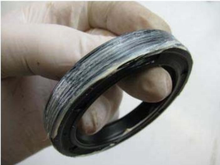
...and I use a bearing race driver and hammer to install it. Go slow with this, and when you strike the seal be aware that you can damage it. A light touch is a good thing. Also, the side cover seal is installed in a somewhat recessed position, but the opposite seal, in the housing, is installed flush with the housing.
