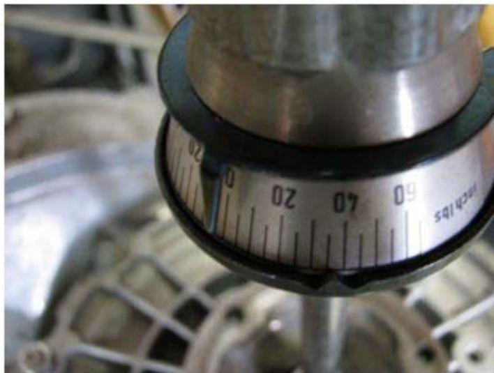
So, what have we learned? I think that the most important aspect of this experiment is that if the thickness of the side cover side bearing is increased, pressure is applied in both directions, and pre-load and backlash are both affected. Therefore, if the differential carrier bearings are replaced, both pre-load and backlash settings become necessary adjustments.
