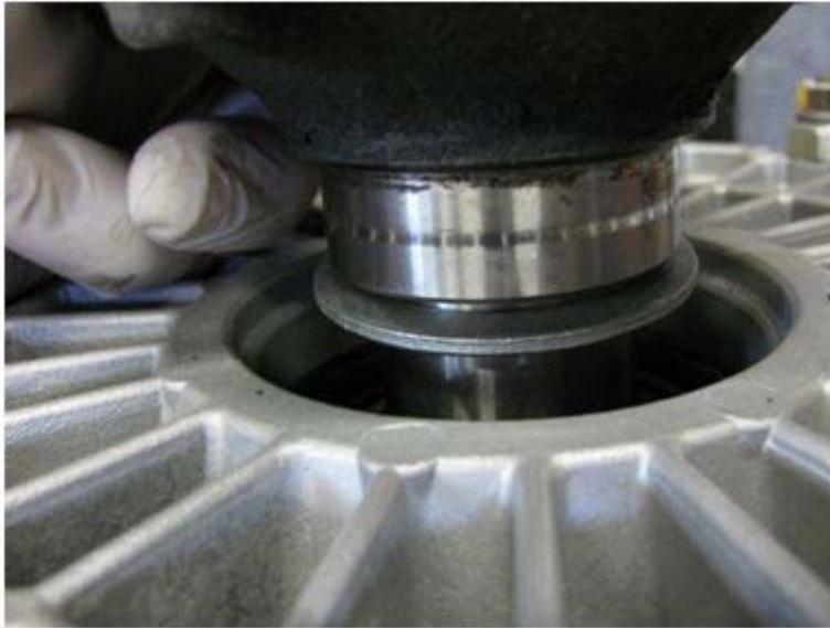
Install the axle flange bolt and hand-tighten it using a socket and ratchet. Install four equally spaced nuts on the side cover, and use them, a little at a time, to “push” the cover into position.
