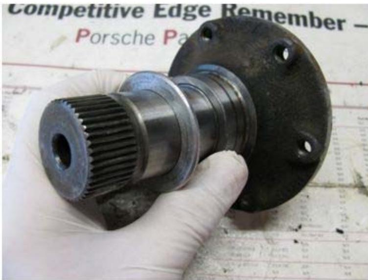
And install the flange through the side cover, into the diff...
