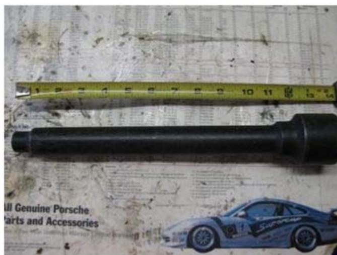
A small version of the dog tooth ring removal tool that we used on 1<sup>st</sup> gear is often necessary, but not nearly as frequent as the 1<sup>st</sup> and 2<sup>nd</sup> gear tool is.
