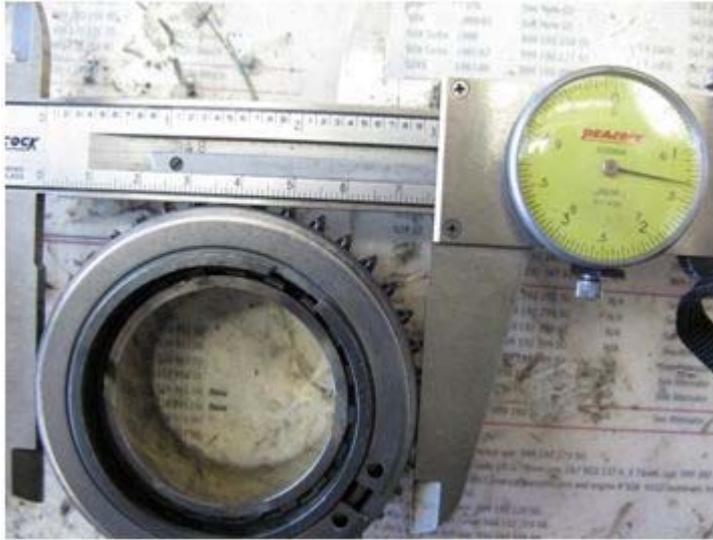
Don't forget to turn the retainer so the opening is away from the opening on the dog tooth ring, and the synchro ring. 3<sup>rd</sup> thru 5<sup>th</sup> gears use the same synchro ring, blocks and bands, and the installed spec (76.3 +/- 0.18mm) is also the same for the three synchros.
