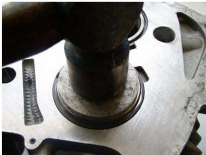
Install the lock ring, and turn it so its gap is at least 90 degrees away from the opening in the housing, and away from the gap in the depth ring. Repeat the entire procedure for the adjacent bearing race, and we can go back to checking detents.
