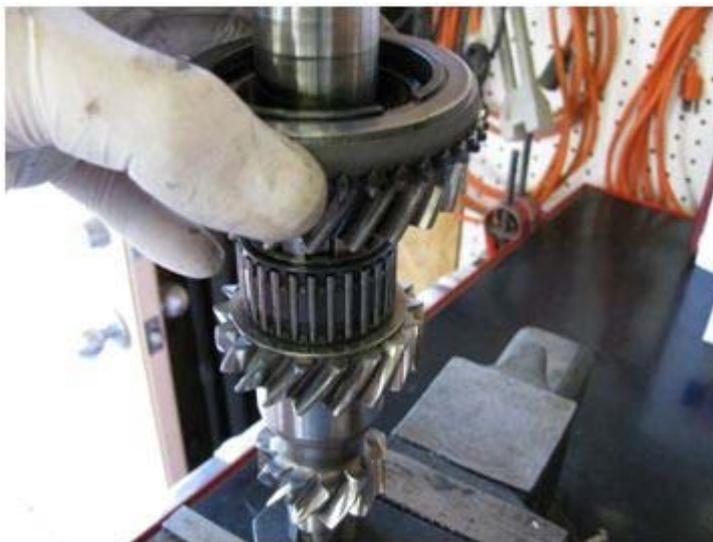
Clean and inspect the slider guide (spider) for 3<sup>rd</sup>/4<sup>th</sup> gear and install it onto the shaft. If your transmission had a big synchro failure, a broken tooth on the spider is possible. If damage (chipping, broken corners, etc.) exists the spider must be replaced. Clean and install your new shift slider; it will probably be coated with an anti-rust product, so soak it in a shallow pan of lacquer thinner in order to clean it.
