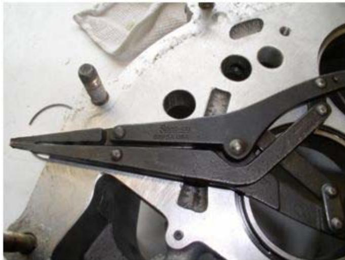
NOTE: Reverse pliers, where the jaws open when the handles are squeezed together, work well for this application.
