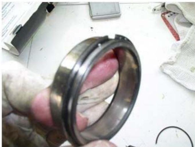
Use an appropriate pliers to spread that ring far enough to work it loose from the bearing race.
