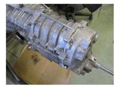
Turn over the transmission, engage the black forks with the shift rod's finger, and move the finger back and forth to make sure it fully engages both forks without hitting anywhere.
