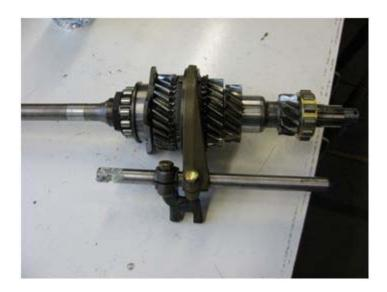
Slide the clutch end of the main shaft into the diff housing, and forward until you can lower the black fork into position on the gear side of the 1/2 fork shaft. At this point line up the two gears of 4<sup>th</sup> speed, and, together, start to push the main shaft and pinion shaft home.
