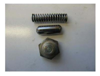
...insert the detent, with a little dab of grease...
