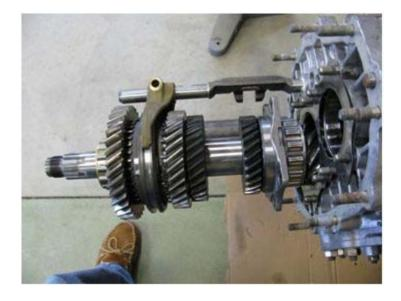
TEST ANSWER: I forgot to install the pinion depth shims, while worrying if my camera had enough battery left for this set of pictures. D'oh!
