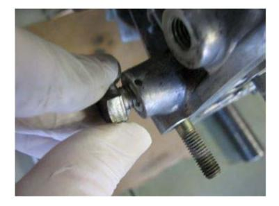
Don't worry; the above picture shows that the plug must be pushed firmly in order to compress the detent spring, and then you have to carefully align the plug with the threads to start it into the opening.
