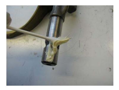
...and slide it into its opening in the differential housing.
