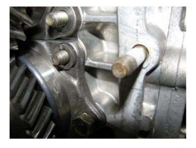
Now we're going to do something that you won't find in the books. Install your P 260A tool onto the main and pinion shafts. I discovered many years ago that by using the P 260A during clamping plate tightening, the pinion and main shafts turn smoother and easier than if they're tightened without the holder in place.
