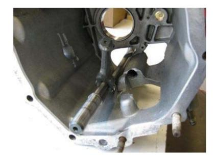
Do the same with the nose cover. Do not use any seals, gaskets or sealant.
