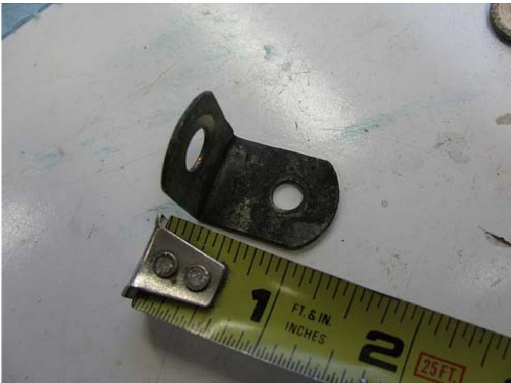
...with or without the remains of a fabric strap attached to it with a 6mm bolt, on the stud above the throttle lever (aka bell crank) mounting pin, discard it. The factory determined, after the fact, that there was no need to have the clutch cable Bowden tube held by the strap/bracket.
