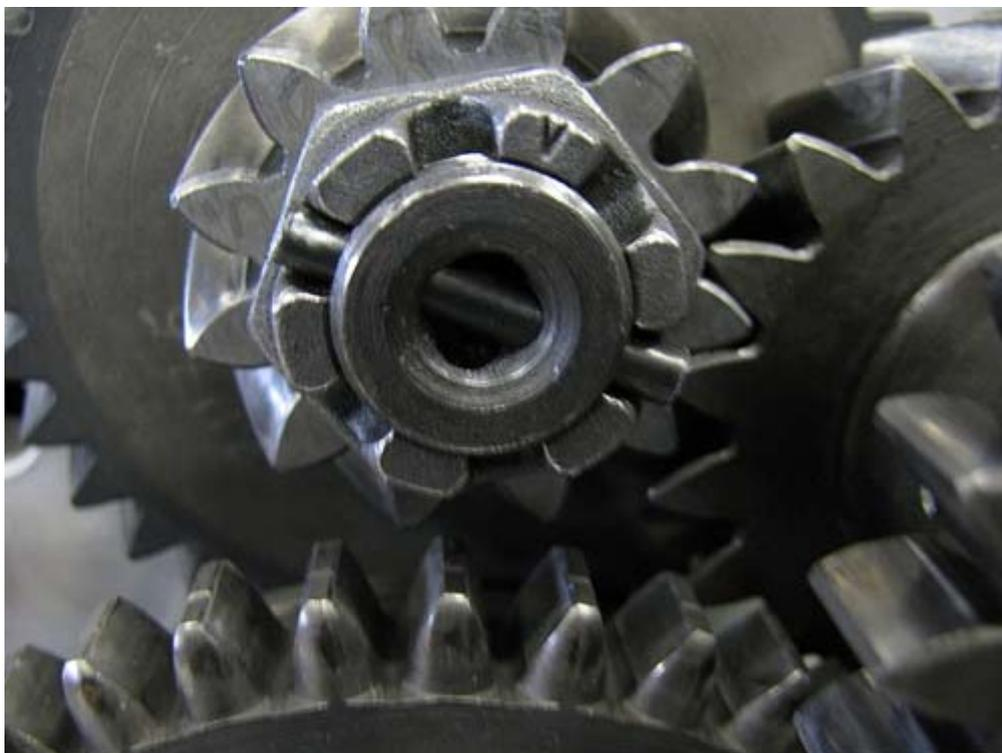
OK, have patience, we're getting close! First we have to check/set the adjustment of the 5/R slider. There is no "middle" for 5/R, so ignore the distance between the slider and the 5<sup>th</sup> gear synchro ring. 5/R adjustment is all about the clearance between the slider and the straight-tooth gear on the reverse idler.
