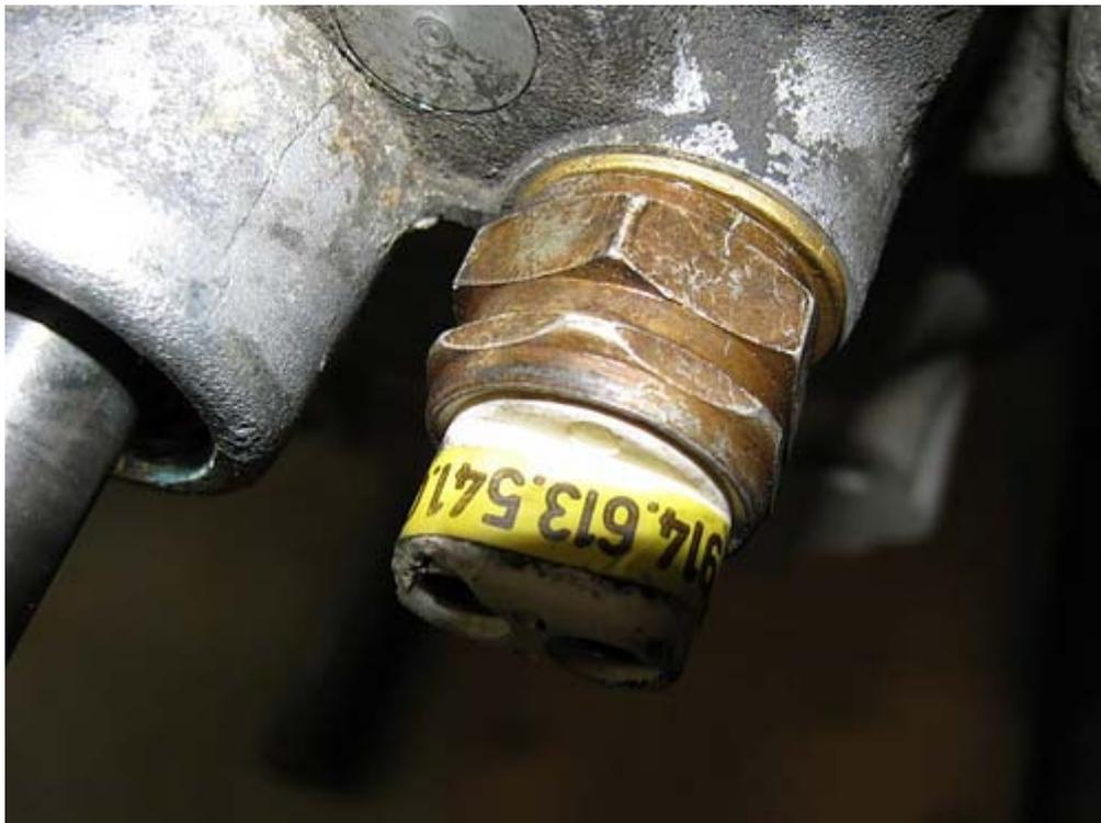
The drain plug is visually the same as the fill plug, except for a small magnet. That magnet should be cleaned thoroughly because it's probably holding onto a lot of debris. Inspect the corners of the plug's in-hex design, if your socket fits nice and snug, re-use the plug.
