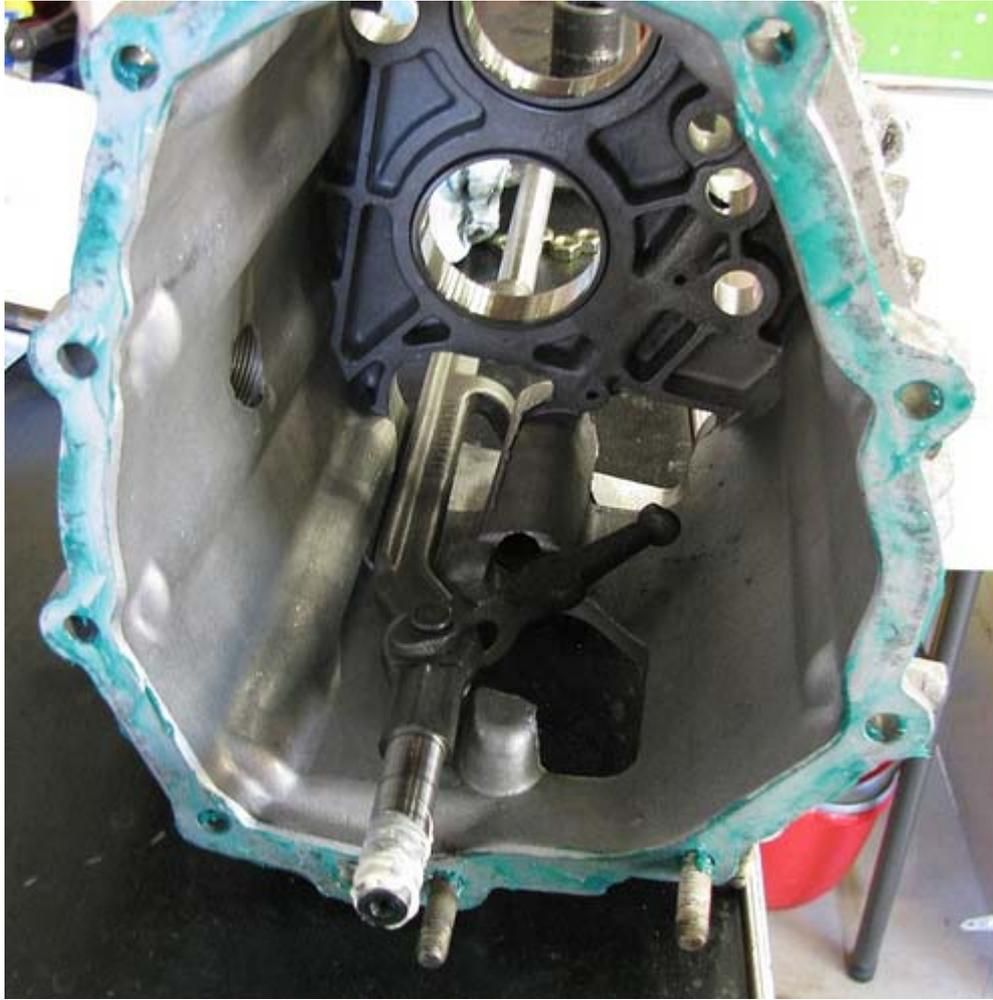
...and put the housing over the gear stack. Check to be sure that the pesky upper detent is where it should be, and begin to push the housing into place. As you get close to the diff housing, push the shift rod into its hole, and get those two lower studs into their holes. You will probably have to turn/wiggle the main shaft and pinion shaft while you're doing all of this, which helps the shaft bearings engage the races in the housing.
