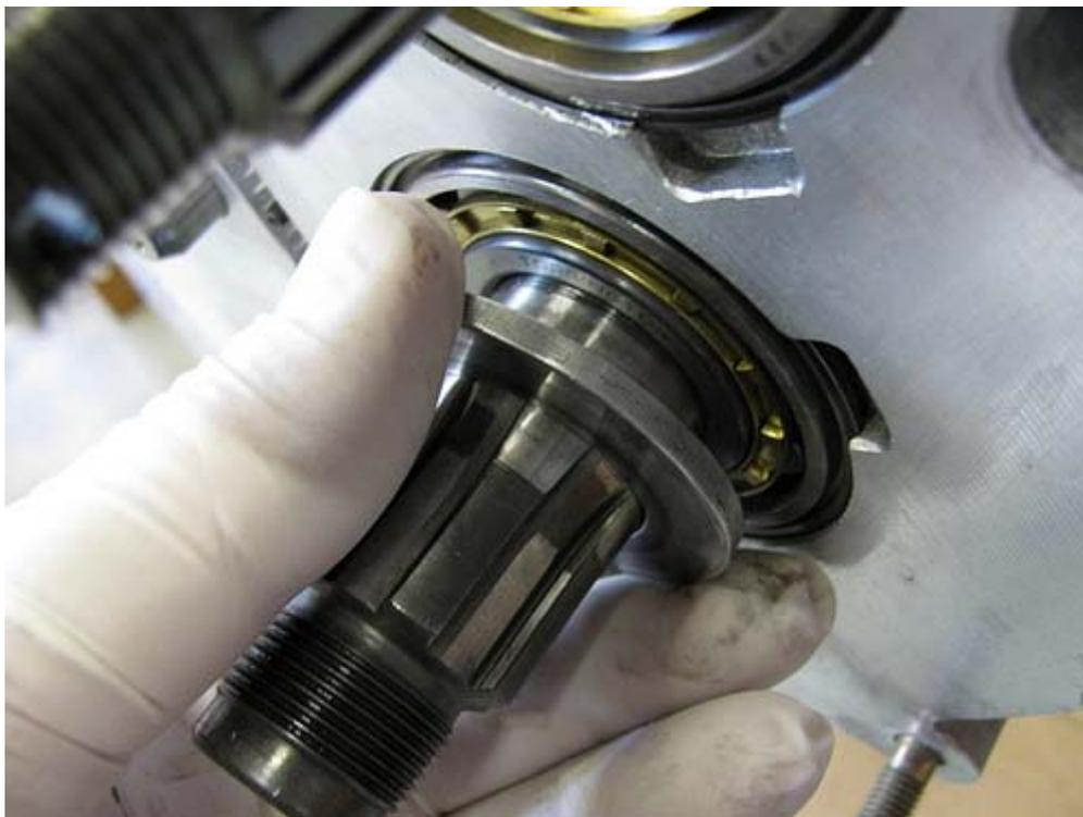
...followed by the 5<sup>th</sup> gear needle bearing and its bushing. Yes, that's a new bearing and bushing, because our almost perfect replacement gear did not include those parts.
