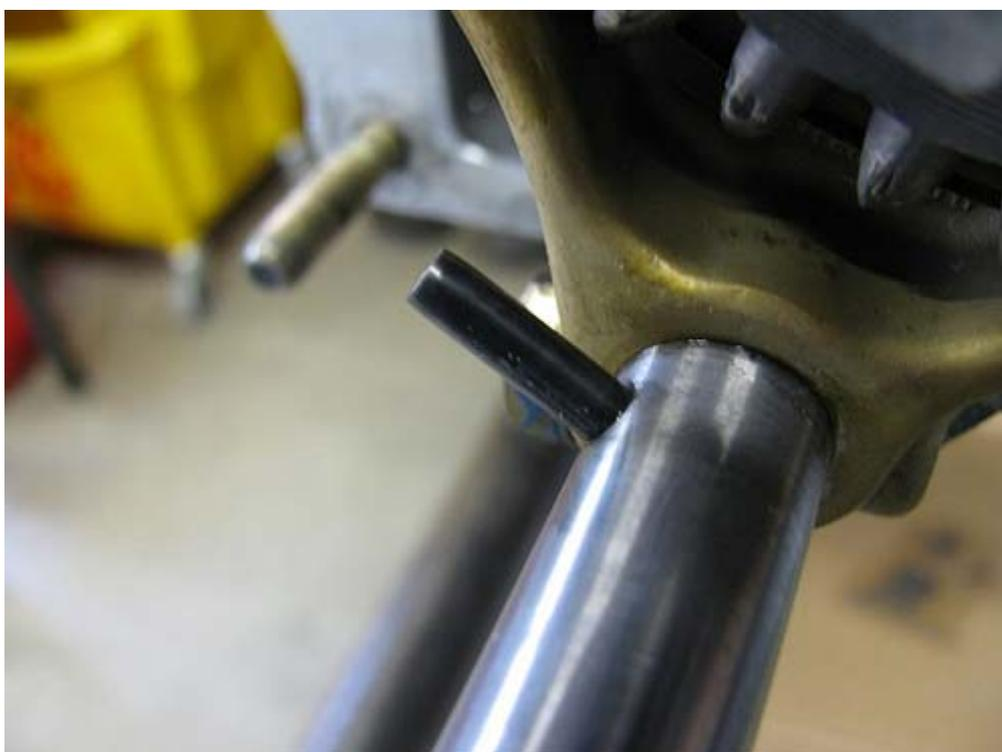
Prepare the nose cover for installation by removing any gasket remnants still on the sealing surface, and then use Q-Tips with lacquer thinner to clean that area as well as the orifice for the shift fork seal. Because there is a chance that someone has replaced the shift fork seal at an earlier time, it is probable that the aluminum recess where the new seal will fit is scarred. We'll do two things to assure a dry nose and a clean
