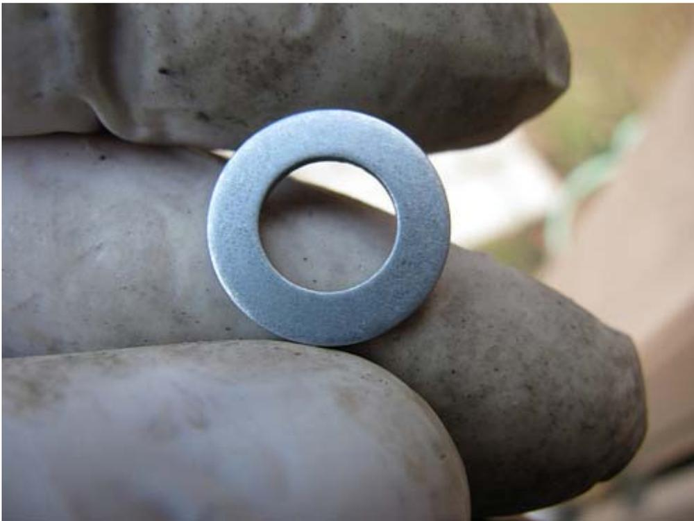
...and will not crush as the required torque spec is reached. Other washers come from Taiwan and who knows where else, have a shiny, silver finish, and are junk. At far less than 18 lb/ft of torque they will crush and collapse into the fastener's threads, which is not what you want to happen.
