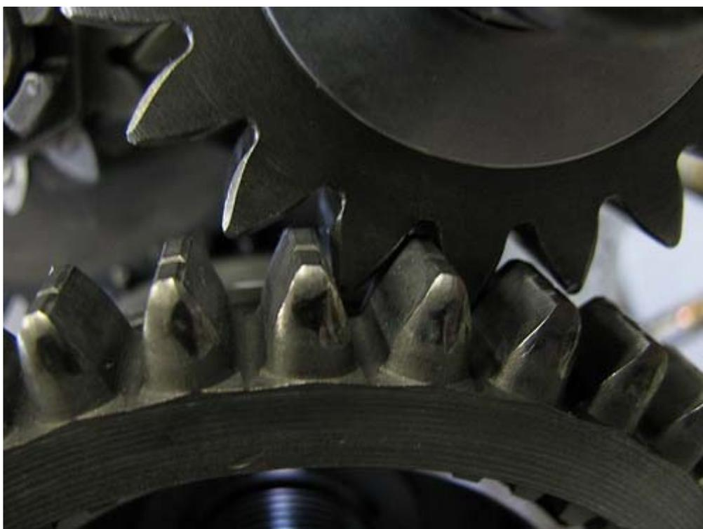
Install your P 37A main shaft lock, engage 5<sup>th</sup> gear, and torque the pinion shaft flange nut to 186 lb/ft. Immediately lock the collar of the nut so you know that it's done. Once again always use new nuts.
