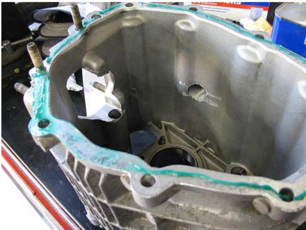
Slide the shift rod into the housing (put a dab of white grease on about an inch of the rod's tip)...
