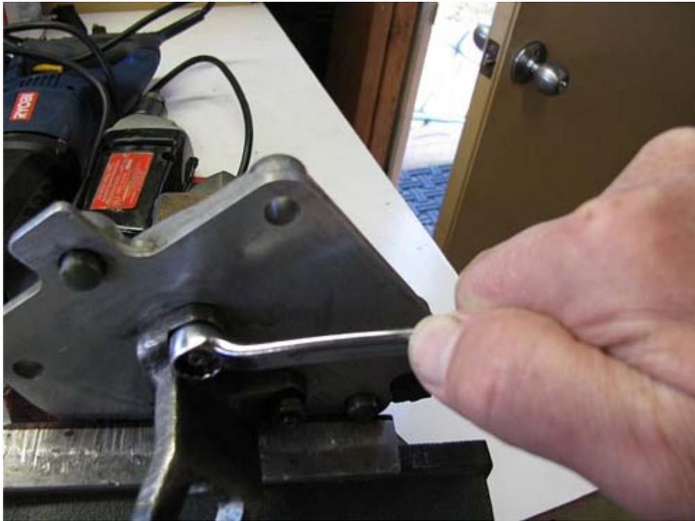
I can't remember ever having to do a thread repair to an aluminum fork plate, but Timeserts work well in this application. With the three nuts tight, Q-Tip the gasket surfaces, apply the Curil T, and install the fork/plate. Use the same combination of sealing washers, wavy lock washers and regular nuts. Torque the nuts to 17 lb/ft.
