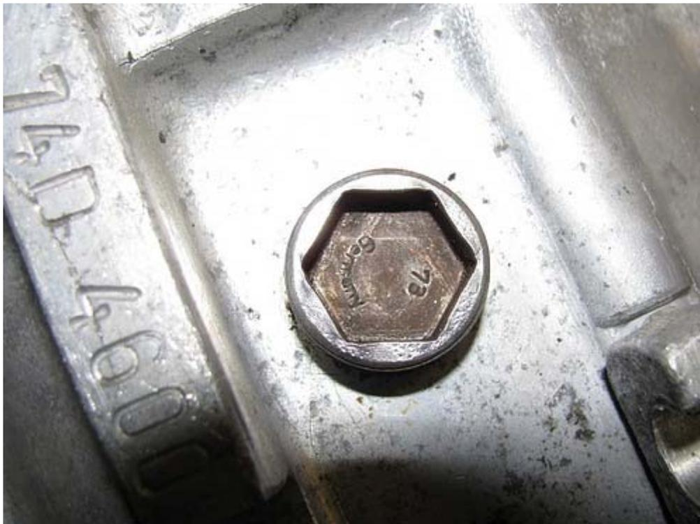
Torque it to 17 lb/ft, and don't use sealing tape, anti-seize, or sealant on its threads.
