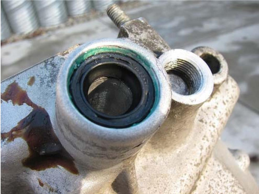
For what it's worth, I use an old 17mm socket that has never been used for anything else, and I ground its end, where it contact's the seal, flat to increase the surface contact area.
