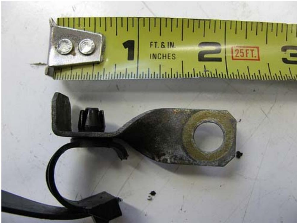
...should be installed. This bracket can be horribly disfigured by mechanics in a hurry to remove the engine and transmission from a car; and the factory wire Ty-rap (shown) is usually cut (shown) rather than released (recommended).
