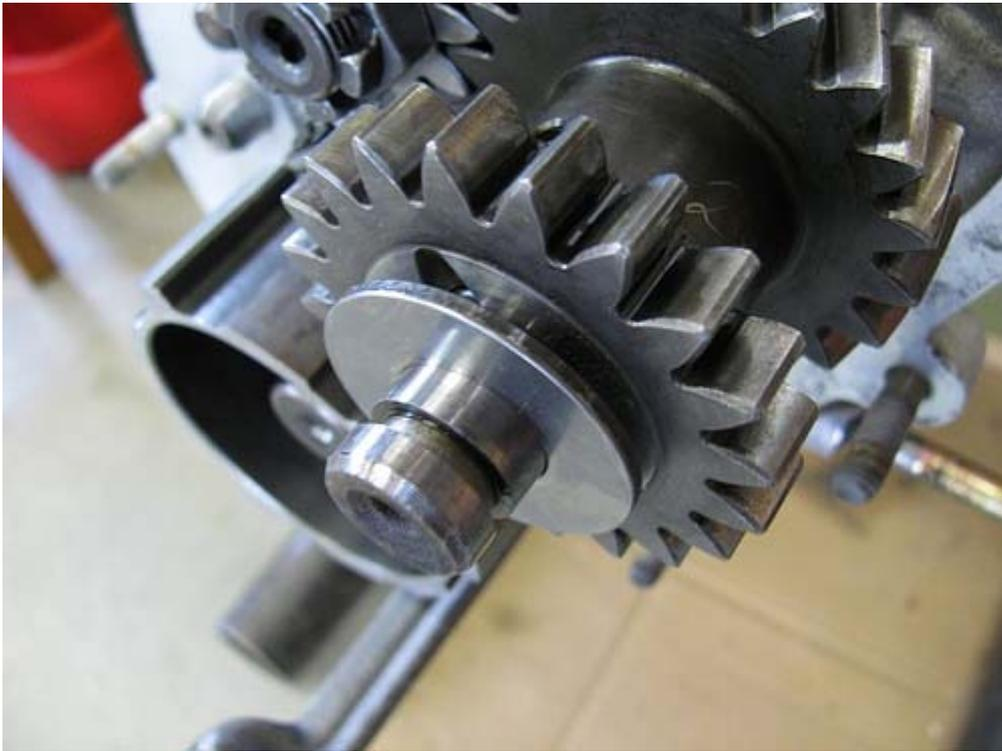
Put the new o-ring from your gasket set into the machined groove at the end of the pin.
