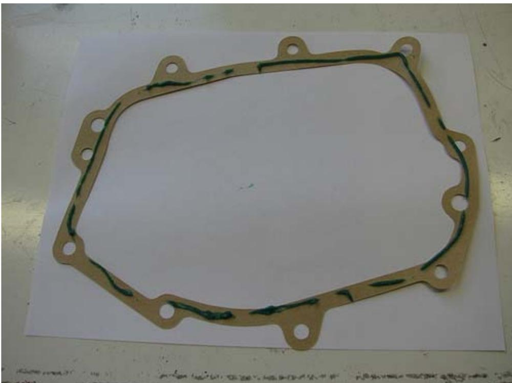
Do the Curil T/O-Tip deal, and gently push the gasket over the studs and press it against the housing.
