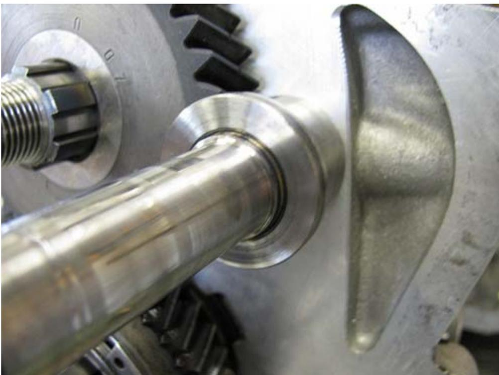
No wear-through of the hardened surface, or tears in the bearing surface, is acceptable. If damage exists on either part, the best thing to do is to replace both, and the flat bearing. Put a dab or two of good quality bearing grease on the idler gear's flat needle bearing...
