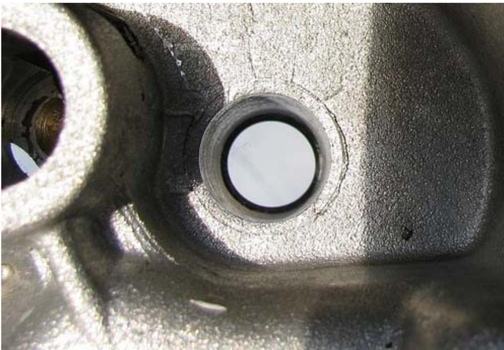
OK, let's install the seal. A driver can be made from wood, metal, or just about anything that you have lying around, as long as it fits inside the seal recess because the seal does not fit flush.
