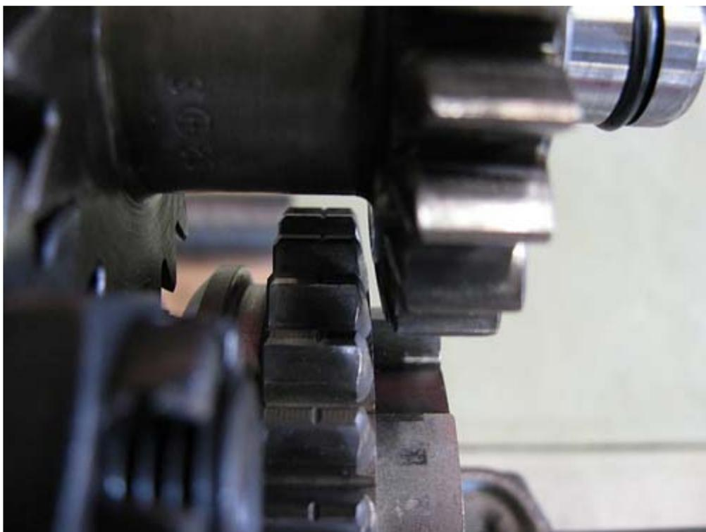
NOTE: If for some reason the reverse switch pin in the shift fork rod was removed, insert it so that about 14mm of the pin projects from the shaft (do this prior to fork/shaft installation).
