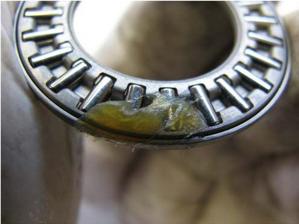
...and slide it onto the idler's pin. The grease will insure that the bearing stays in position during assembly (it can hang up on the pin's shoulder and make a mess out of everything). Install the pair of idler bearings, with their spacer ring in the middle.
