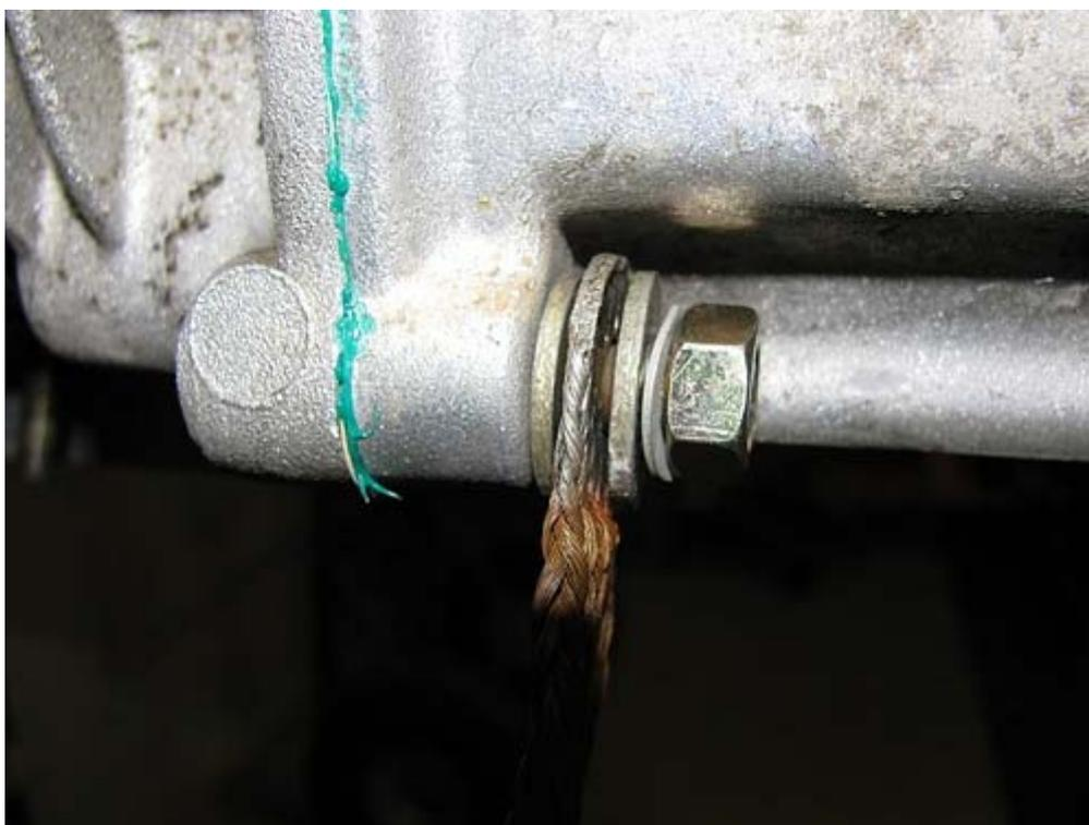
The correct installed position for the strap is straight out to the right (driving direction) side.
