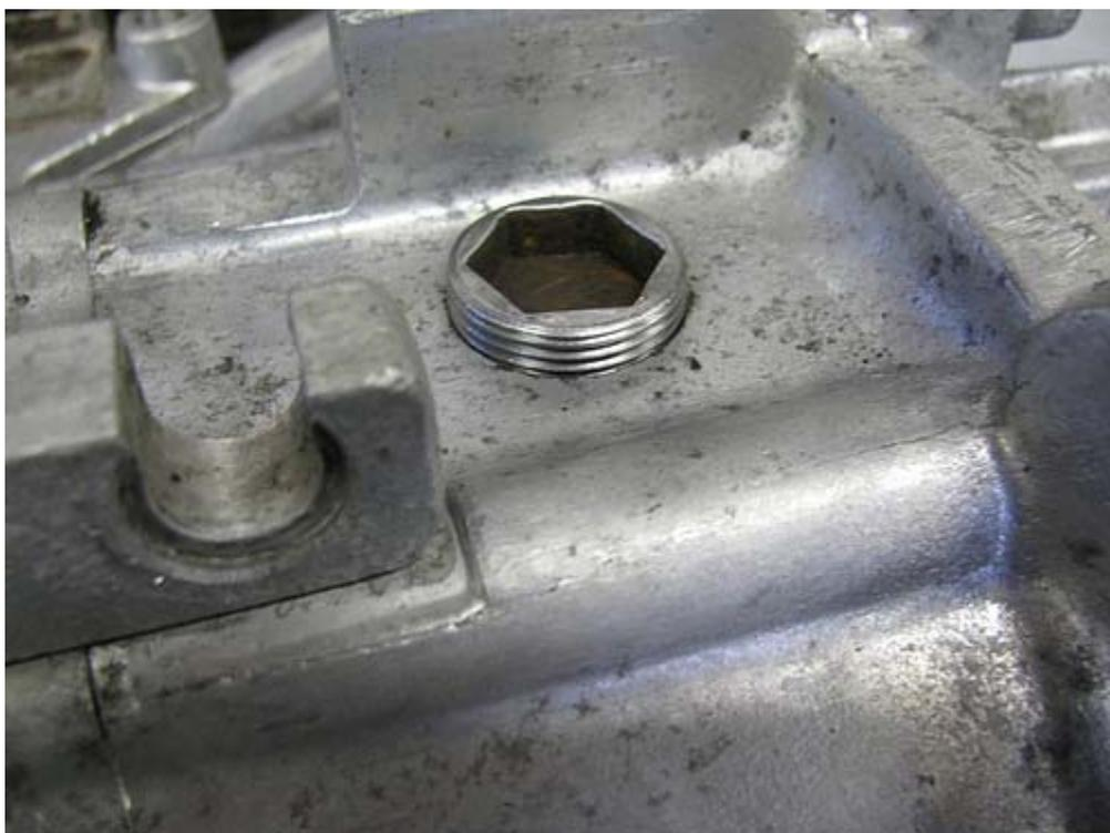
NOTE: If the transmission is scheduled for immediate installation and use, I don't install the fill plug until after the transmission has been filled. If it's put into storage, I insert the fill plug a couple of threads, and tag the unit with a reminder to fill it at installation.
