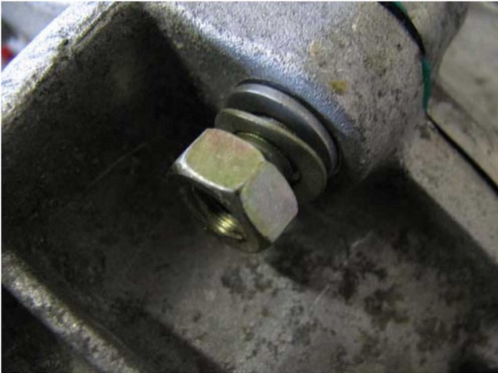
As was the situation with the clamping plate nuts, unless you own a Stahlwille torque wrench set that can torque fasteners that a mere mortal wrench can't, tighten the nuts in a crossing pattern until they're all snug. Use the box end of your end wrench and try to get each nut as close to 17 lb/ft as possible. If necessary, practice some more using that bolt and nut that we had in your vise.
