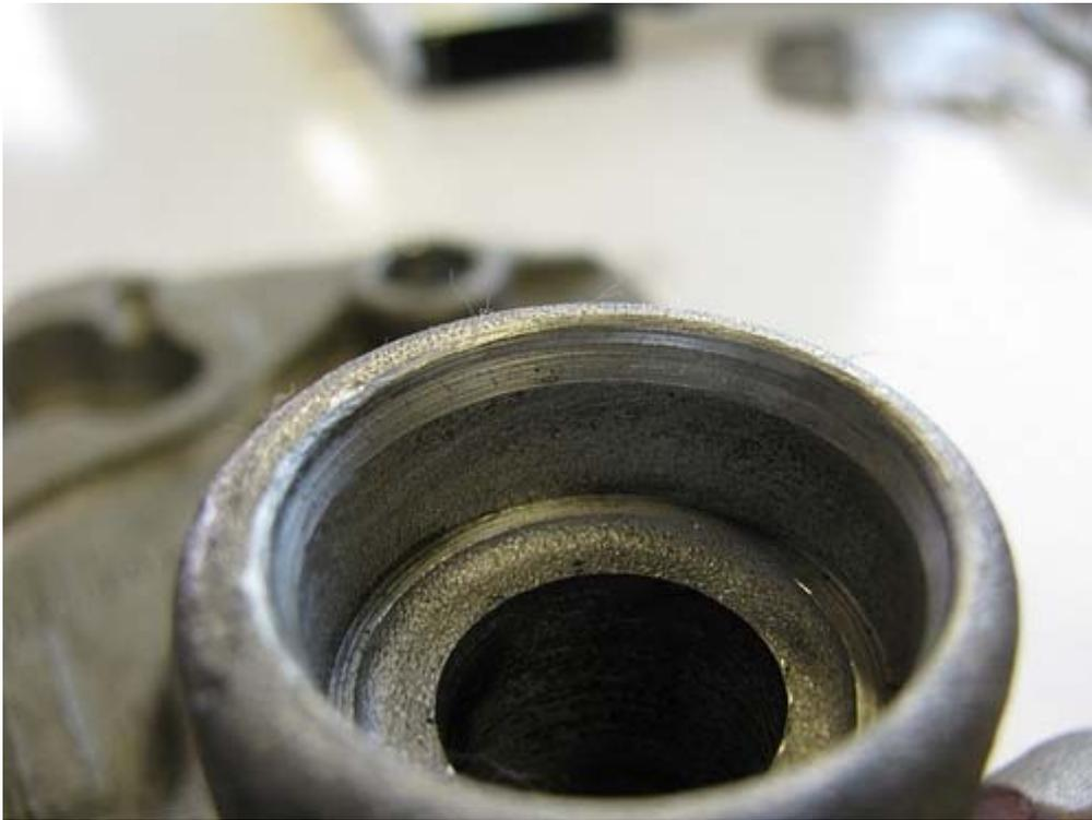
Hold the seal so that you can put a very thin layer of Curil T on the outside surface of the seal, and then push the seal into place. The sealant will offset any small imperfections in the aluminum, and create a seal that will prevent trans oil from escaping around the outside of the seal.
