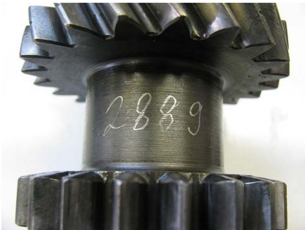
Before going further, carefully examine the bearing surface at the end of the idler, and the corresponding surface on the idler mounting pin.
