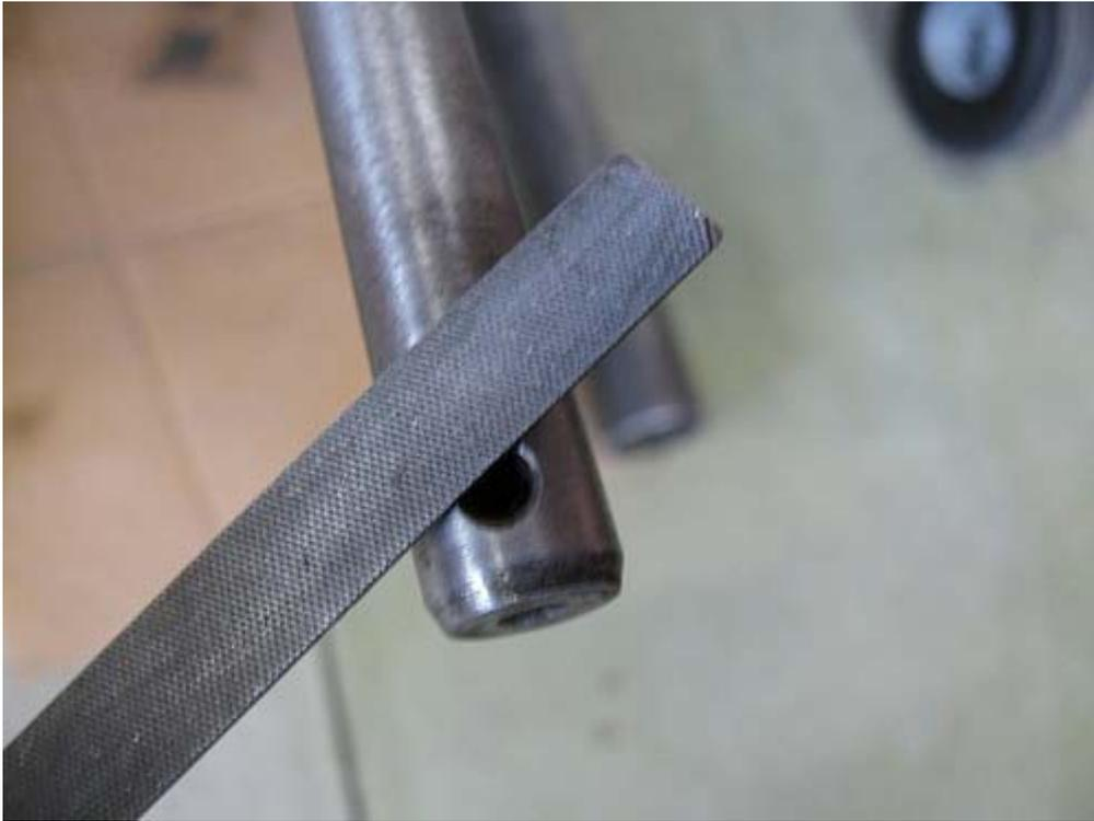
...or emery paper, to clean away any rough edges, and then apply a thin coat of white grease to the tip of the rod. Add additional grease to the o-ring on the reverse idler mounting pin. Clean the gasket surface one more time, with lacquer thinner and Q-Tips, and apply Curil T. Install the nose cover. A gentle push, maybe a little tap with the heel of your hand to engage the idler pin's o-ring, is usually all that's necessary to seat the cover against the center housing.
