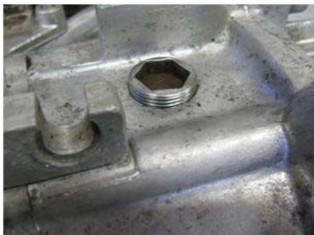
The change was done, as close as I can pin-point it, at the end of 915/61 production. If ever in doubt, use 17 lb/ft as the torque spec, no matter if your transmission has a magnesium, or aluminum, housing, or if your plugs are the early or late type.
