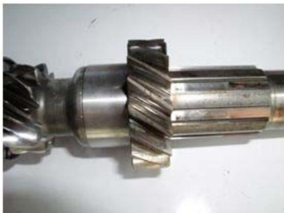
So, for many years, I've used the 166 lb/ft torque spec for all late main shafts, and use the high side of the early torque spec for early style main shafts.
