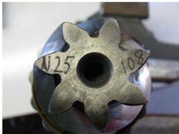
...that is actually the "r" number. "r" is the number that is the deviation (the distance deviating from design distance "R") that is measured by the factory. "R" is a set number, and is the distance between the center of the ring gear, and the inner edge of the ring gear's usable gear teeth. On 915s "R" = 66.30mm, and the gauge block (micrometer) is used to compress the contact plunger...
