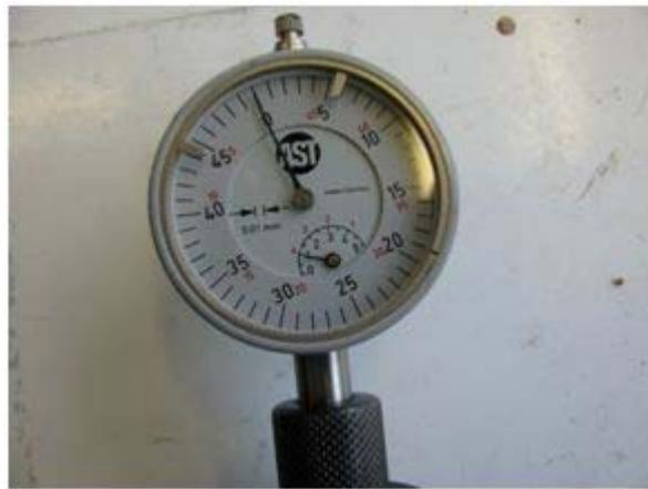
...may be set to 1mm pre-load so that the actual position of the pinion head, without shims, can be measured.
